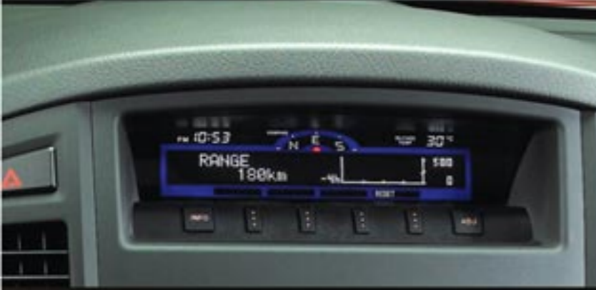
• Multi-Information Display Monitor (Function Customizer, Compass, Outside Temperature, Drive Computer, Fuel Economy, Digital Clock, Altitude Display, Air Conditioner Info)
